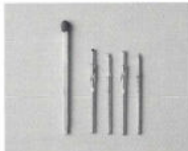
Fig. 5: Exchangeable and gilded contact pins
