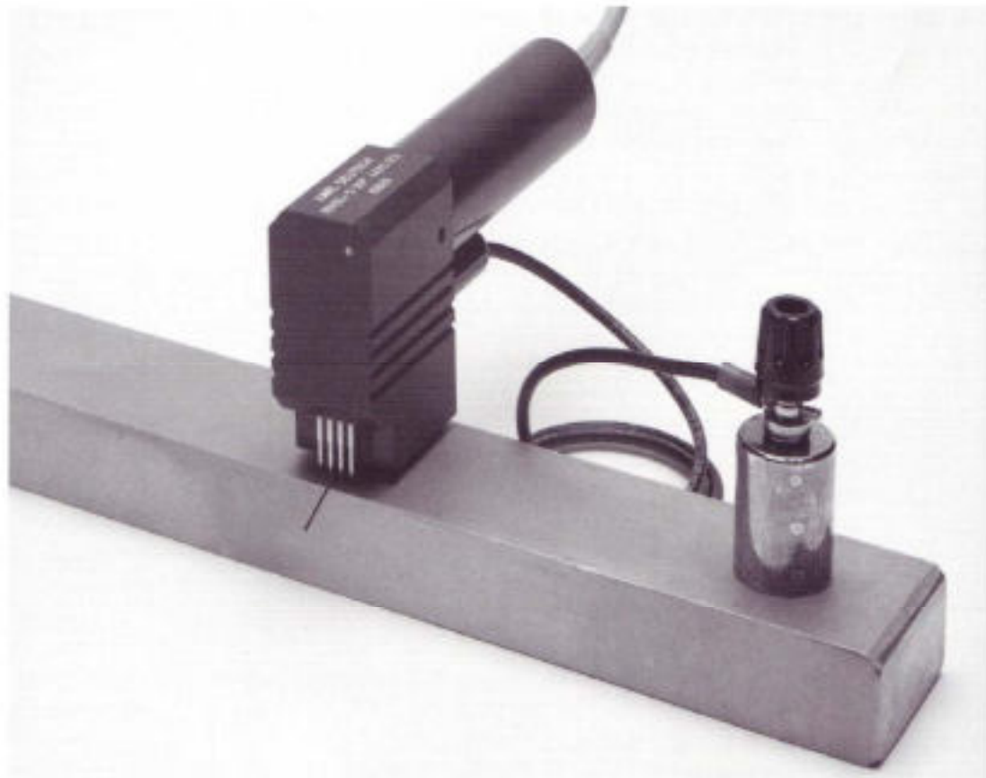
Fig. 7: Special probe to measure inclined cracks
