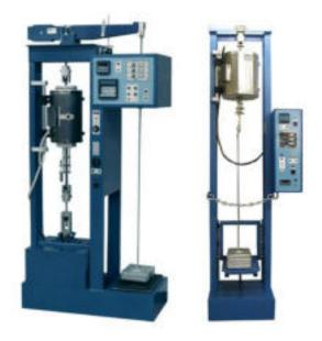
Lever arm and direct load test frames, any number and in any combination, from any manufacturer, can readily be adapted to suit the WinCCS II system. WinCCS II can also be supplied as an integral part of a new ATS creep testing installation.
