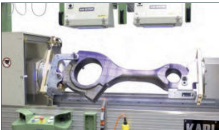
Testing of connecting rods for ships. Motor-driven face plates for the rotation of the workpiece inside the machine during the visual inspection. Pneumatically movable UV lamps.
