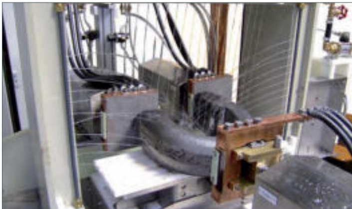
Special machine with three contacts (3000 A each) for the testing of chain bows.
