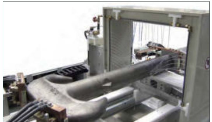
Flexible angle and distance adjustment, here for testing of double hooks.
