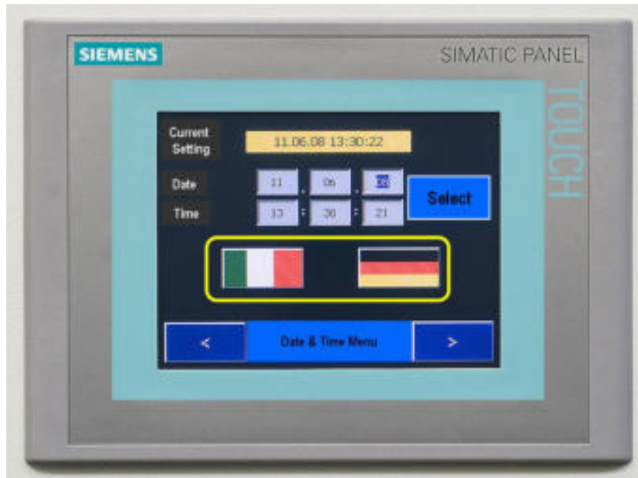
Figure Switch-over of Language. Comfortable operation in native language by electronic switch-over
