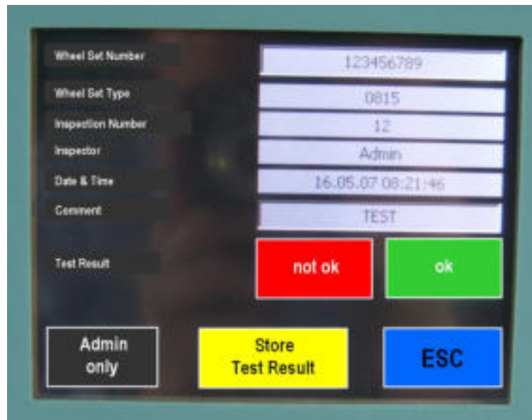
Figure Test Parameter for Railway Axles. Important test parameters are stored within the test protocol. The most important information namely the test result has been highlighted by colour in the operation mask.
