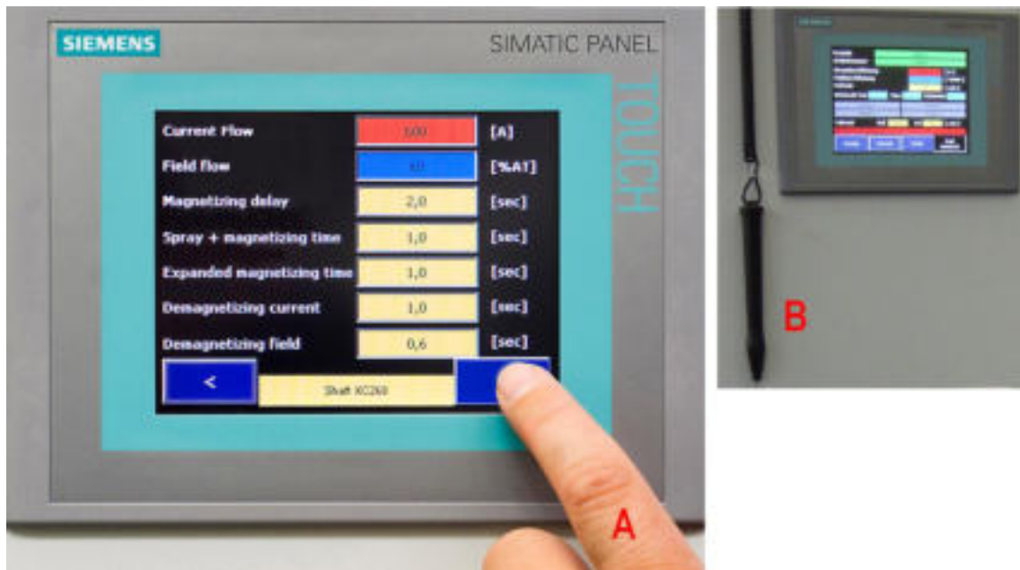
Figure Touch Panel. Operating panel of the parameter store with input by hand (A) or by pen (B).
