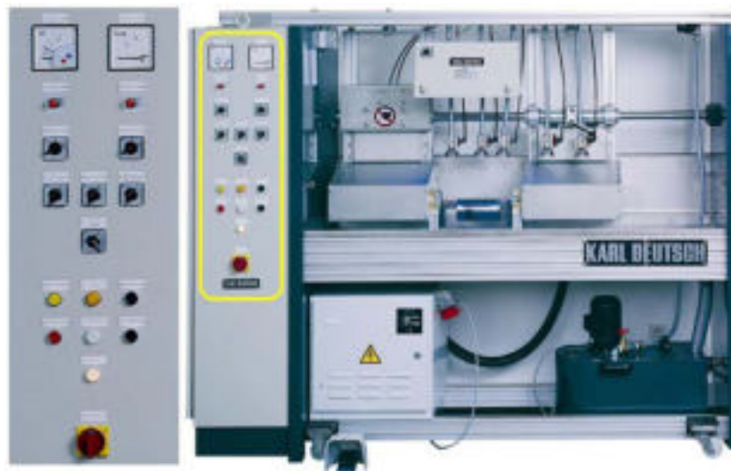
Figure Test Machine with 2 Contacts. Universal test bench with 2 magnetization circuits and conventional electrical control.
