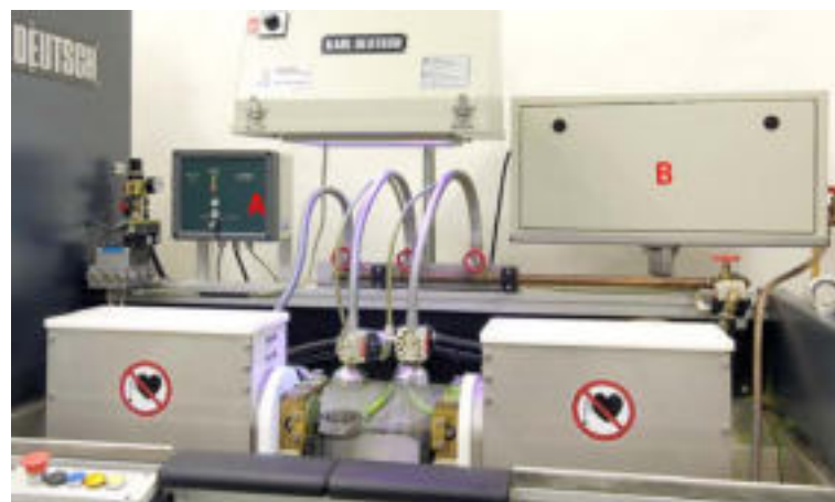
Figure Test Machine with Crack Test Liquid Control Unit. The operation and display module (A) indicates via coloured bar-graph representation the quality of the crack test liquid. The measurement module (B) is also mounted directly to the machine.
