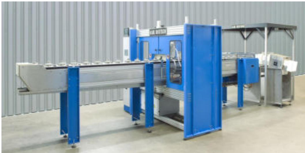
Figure Machine with Chain Conveyor. The components (wheel hubs) are fed from left to right through the encapsulated test machine. The parameter storage serves not only as control unit of the testing process. The proper position of the chain is monitored and is corrected if necessary. At the inlet of the test machine light barriers are mounted for checking the loading state. The transport and the testing process are only started when the chain is completely filled. At the outlet the observation cabin is shown (still without curtain).
