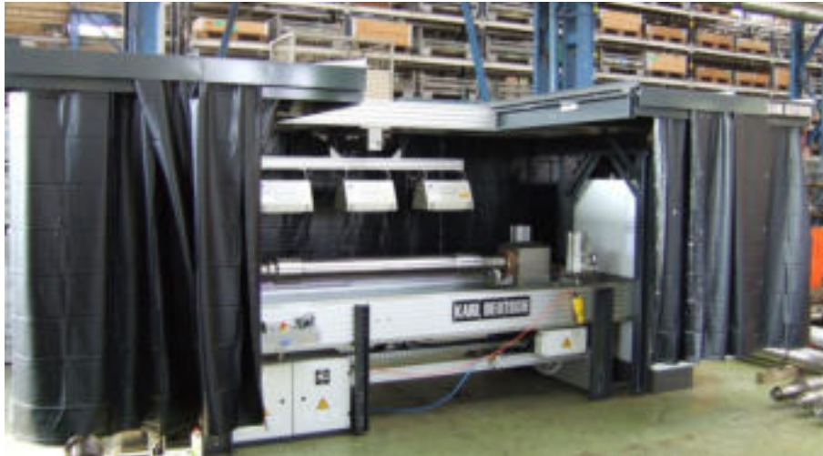
Figure Axle Testing. Test machine to check railway axles with test cabin. The roof can be opened pneumatically which allows loading by crane.
