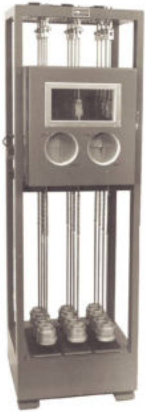
Series 2120 Direct Load Creep Tester with special 12-station configuration. Environmental chamber includes hand access ports.
