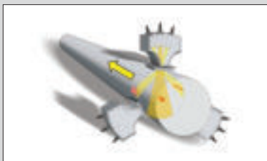
Testing of (e.g. black) bars with 9 probes in 3 probe holders
