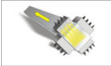
Testing of quadratic billets with 28 probes in 4 probe holders
