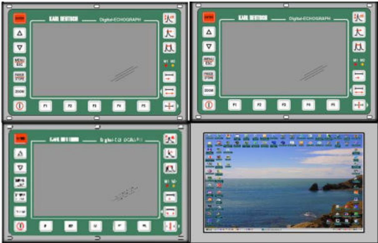
Figure 2. Ultrasonic electronics with three channels and a host-PC. All modules are mounted into a 19" rack (in this example with a total height of 13 units).
