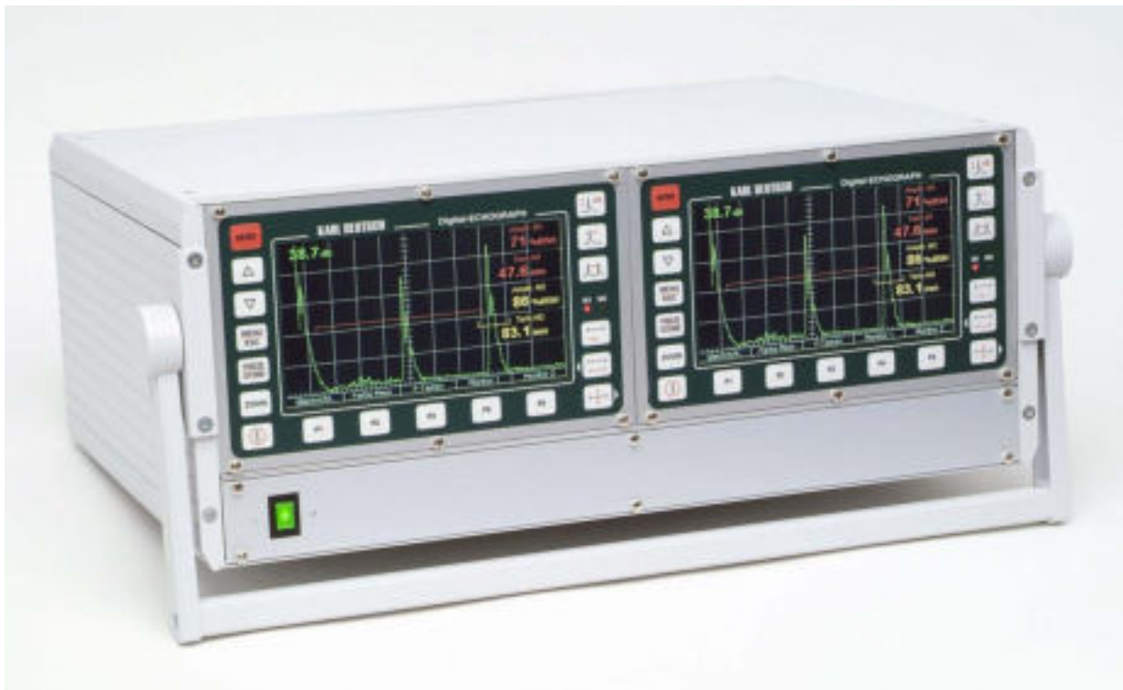
Figure 1. Two-channel setup of ECHOGRAPH 1092 with a carrying handle. Two gates are active for each module (red and yellow horizontal bar). The corresponding measurement values (e.g. amplitude and flaw depth) are shown on the right side of the A-scan in large letters. The colours of the measured values correspond to the colours of the gates. A main power switch is provided for the rack-mount instrument.
