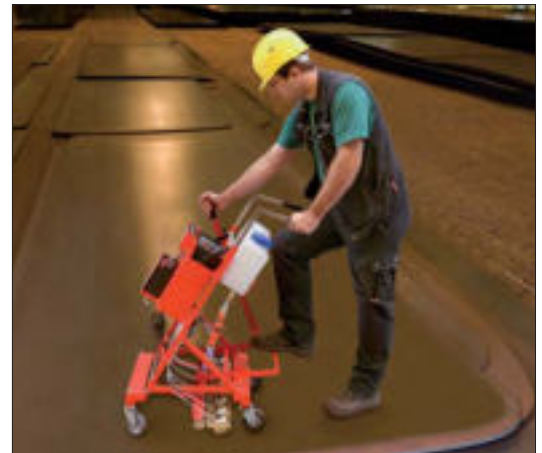
Ultrasonic testing on sheet metal by trolley (8 test channels)
