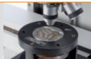
Microhardness determination on a polished microsection
