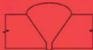
74 Excess Crown in Single Vee, VT
