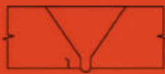
19 Base Metal Crack in Single Vee (bottom HAZ area) MT/PT, UT
