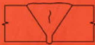
15 Centerline Crack, Single Vee (sub-surface) UT, RT
