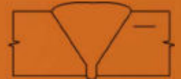
50 Lamination in Single Vee (base metal) UT
