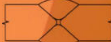
57 Incomplete Root Penetration in Double Vee, UT, RT
