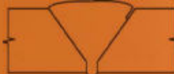
53 Lack of Fusion in Single Vee (surface breaking at crown) MT/PT, UT
