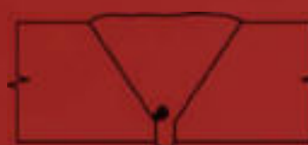
36 Slag Inclusion in Single Vee (root area) UT, RT
