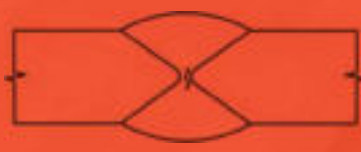
15 Centerline Crack in Single Vee (sub-surface) UT, RT
