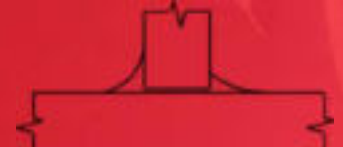
73 Uneven Leg Length in Fillet, VT
