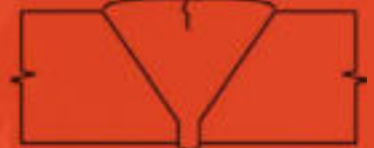
14 Centerline Crack, Single Vee (surface breaking) MT/PT, UT, RT
