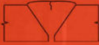
11 Toe Crack in Fillet MT/PT, UT
