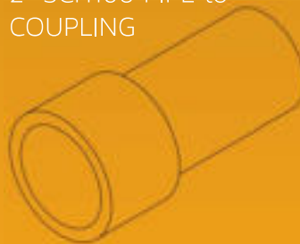
P109 WELDED PIPING 4" SCH160 (0.53" T) x 8"
