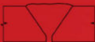
71 Excess Root Penetration in Single Vee VT, RT
