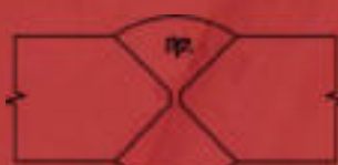
30 Porosity in Double Vee (sub-surface) UT, RT
