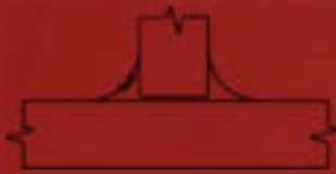
33 Porosity in Fillet (surface breaking) VT, MT/PT
