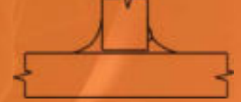
54 Lack of Fusion in Fillet (surface breaking at crown) MT/PT
