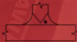
38 Slag Inclusion in Fillet (root area) UT, RT
