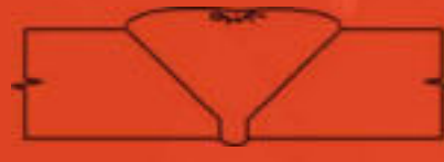
20 Crater Crack (crown stop-start area) MT/PT, UT
