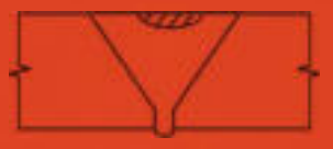
17 Transverse Crack in Single Vee, flush crown MT/PT, UT
