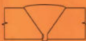
55 Lack of Fusion in Single Vee (surface breaking at root) MT/PT, UT
