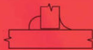
75 Excess Crown in Fillet, VT
