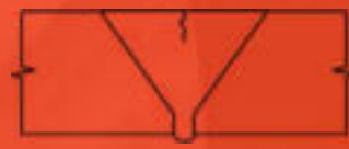
16 Circumferential Crack in Single Vee, flush crown MT/PT, UT
