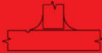
79 Undercut in Fillet, VT
