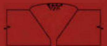
32 Porosity in Single Vee (surface breaking) VT, MT/PT
