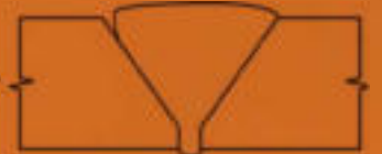
59 Incomplete Groove Weld (crown area) VT, MT/PT, UT, RT
