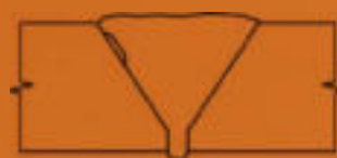
52 Lack of Fusion in Single Vee (crown area) UT
