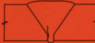
12 Root Crack in Single Vee MT/PT, UT, RT
