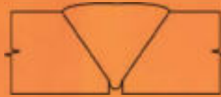
56 Incomplete Root Penetration in Single Vee, VT, UT, RT
