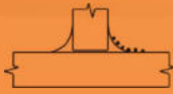
91 Weld Splatter on Filler VT, RT
