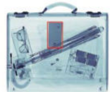
Example of DEXGIL automatic explosive alert in an apparently innocuous luggage
