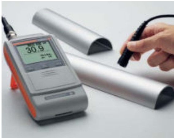
DUALSCOPE® FMP20 with anodized parts. Measured using a curvature-compensated probe (Fischer patent).
