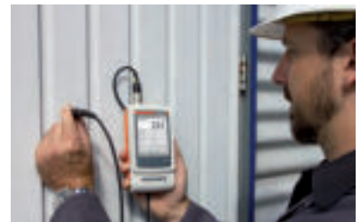
Measurement of paint coating thickness
