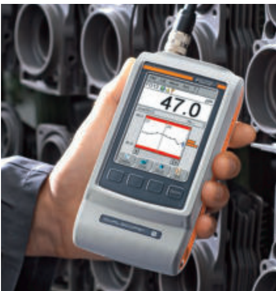
Graphical display of the measurements with the set specification limits. The histogram of the measurements is additionally shown on the right display site.
