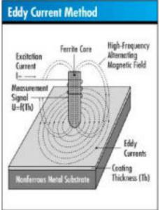
digital reading. Common applications include liquid or powder coating over aluminium and nonmagnetic stainless steel, and anodize over aluminium.
