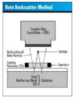
coating thickness. Reliable applications for the beta backscatter method are measurements where the atomic number of the coating and substrate differ by 20 percent. These include gold, silver or tin on electronic components as well as coatings on machine tools, decorative plating on plumbing fixtures, and vapour-deposited coatings on electronic components, ceramics and glass. Other applications could include organic coatings such as oil or lubricant over metals.
