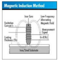
This method is quick and can be used with either a bench top or hand-held coating thickness gage. Common applications include liquid or powder coatings, as well as plating's such as chrome, zinc, cadmium or phosphate over steel or iron substrates.
