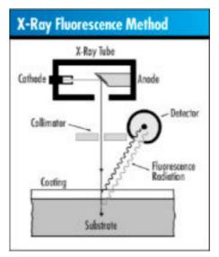
X-ray fluorescence isn't used to measure organic coatings. It's also somewhat limited by the coating's thickness, usually not exceeding 0.5-0.8 mils. However, unlike the beta backscatter method, X-ray fluorescence can measure coatings with similar atomic numbers, such as nickel over copper. Different geometrical parts can also be measured with this method.
