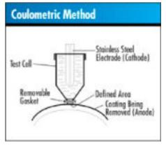
surface area are constant, and thus the coating thickness is proportional to the time it takes to strip the coating. This method is particularly useful for measuring electrically conductive coatings on a conductive substrate.
