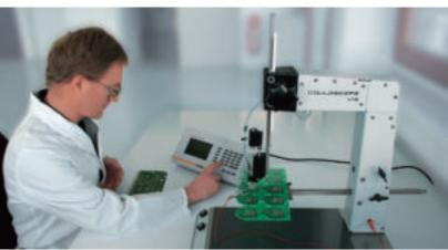
▲ COULOSCOPE<sup>®</sup> CMS: Determination of the remaining tin thickness on electroless tin-plated PC boads.
