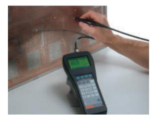
▲ PHASCOPE<sup>®</sup> PMP10: Determination of copper coating thickness on non-etched or etched PC boards and determination of copper coating thickness in bore holes.
