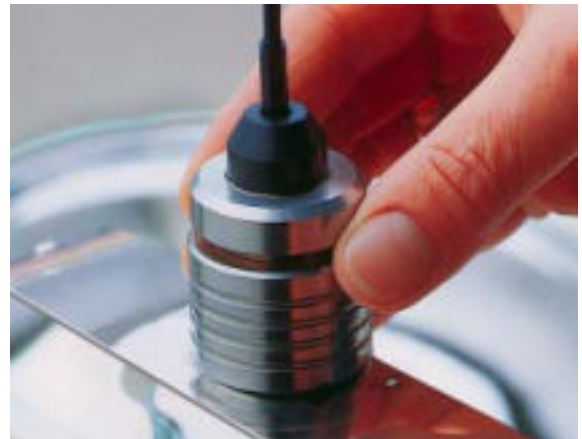
Fig. 9: Betaprobe Z9NG, Pm-147 isotope, 1,6 mm aperture on CdTe-panel
