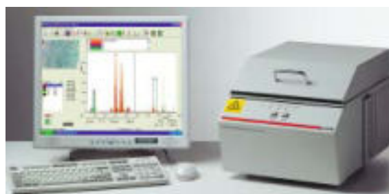
FISCHERSCOPE® X-Ray XAN-DPP Spectrometer for quick analysis of small CIGS objects in the quality lab (manual table)
