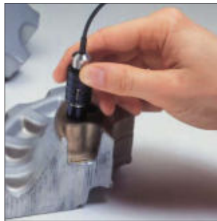
Measurement of an anodic coating on aluminum components using the probe ETA3.3 according to the amplitude sensitive eddy current method.
