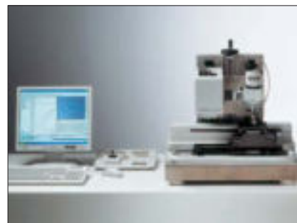
Microhardness test instrument FISCHERSCOPE® HM2000 for testing the hardness according to ISO 14577.
