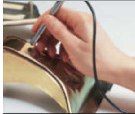
Measurement of zinc coatings using the probe EGAB1.3 according to the magnetic induction method.
