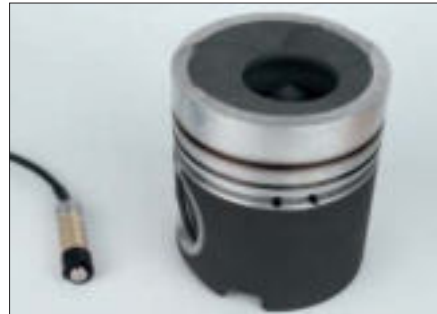
Measurement of the nickel coating thickness on a piston using the probe EN3 according to the magnetic method.
