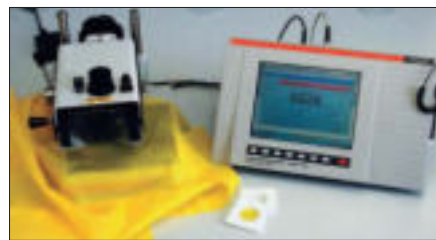
Inspection of the homogeneity of a screen-print fabric after calendering using the measuring stage Z6NG.
