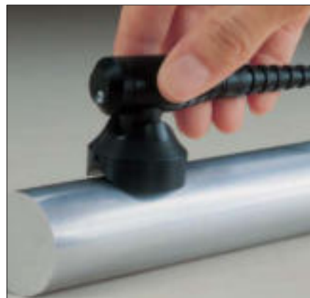
Measurement of the electrical conductivity of aluminum components for testing the strength using the probe ES40.
