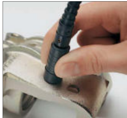
Measurement on rough surfaces, e.g., Zn/Fe, using the probe ESD20Zn according to the phase sensitive eddy current method.
