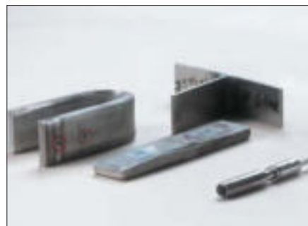
Measurement of the ferrite content using the probe EGAB1.3-Fe according to the magnetic induction method.
