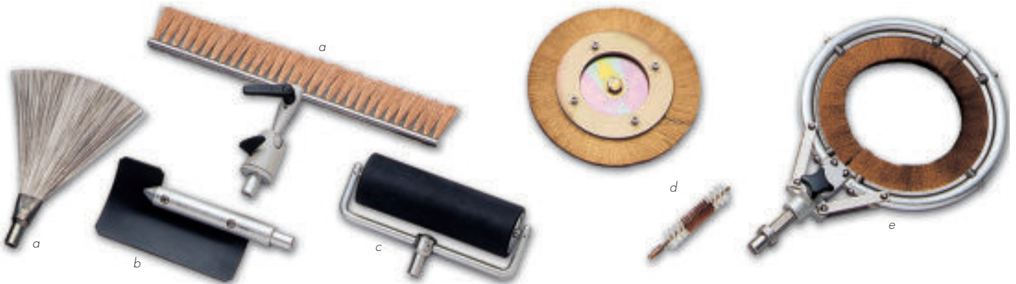
Overview of the various electrodes: a) Sweeper electrode b) Flat electrode c) Roller electrode d) Rotating electrodes for tests inside pipes e) Circular ring electrode for tests on the outside walls of pipes
