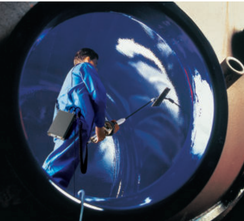
Porosity detection in the Enamel coating of a Kettle with the POROSCOPE®
