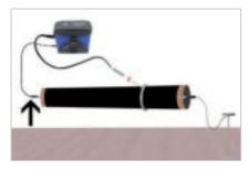
**Direct grounding -** The directly conductive connection between the testing instrument and the not-insulated section of the pipe to be tested is the most reliable form of grounding, and is to be preferred to all other options.
