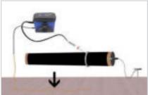
**Indirect grounding** with the help of the trailing ground enables pipeline testing without obstructing cables, if direct grounding is not possible.
