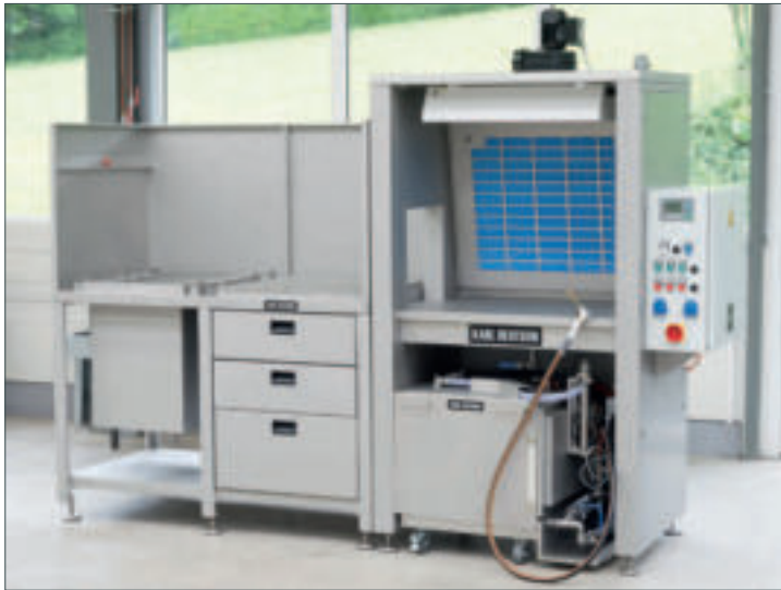
Test station for laboratory with dip tank and drawers
