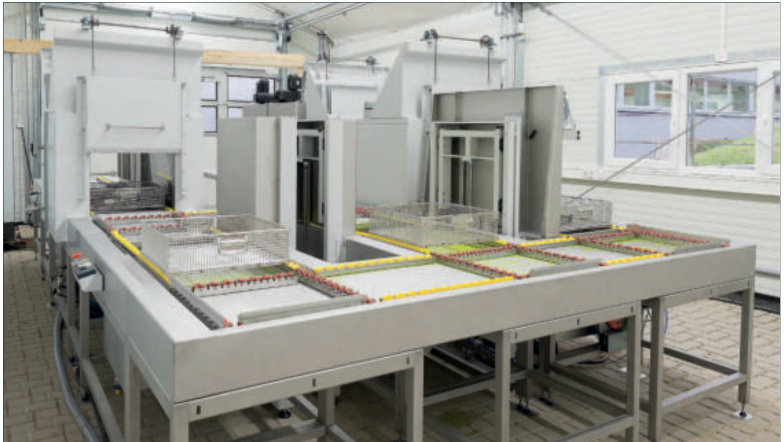
Semi-automated testing system with pre-cleaning unit and two dip tanks for penetrants of different sensitivity.
