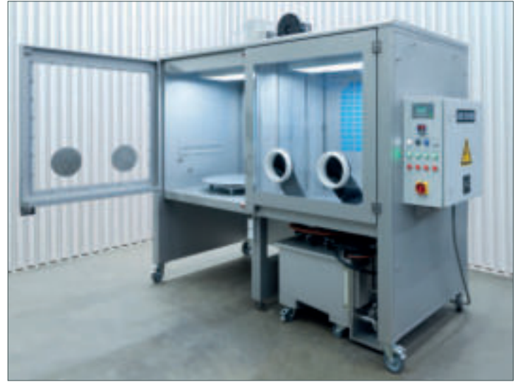
Customized testing station with splash protection doors and integrated drying facility
