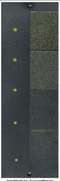
test block no. 2 according to **DIN EN ISO 3452-3**
