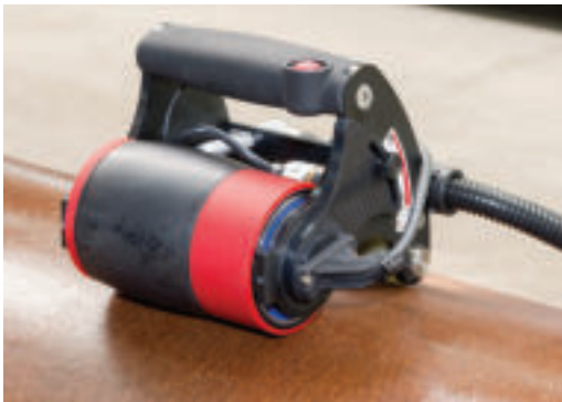
Roller probe for circumferential testing of bars and tubes
