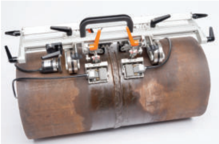
Scanner for manual testing of circumferential tube welds with position encoder and suspensions for 2 Phased Array probes and 2 TOFD probes
