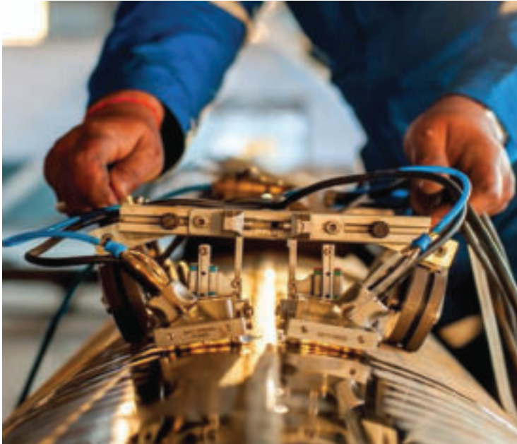
Scanner for manual testing of longitudinal tube welds with position encoder and suspensions for 2 Phased Array probes and 2 TOFD probes
