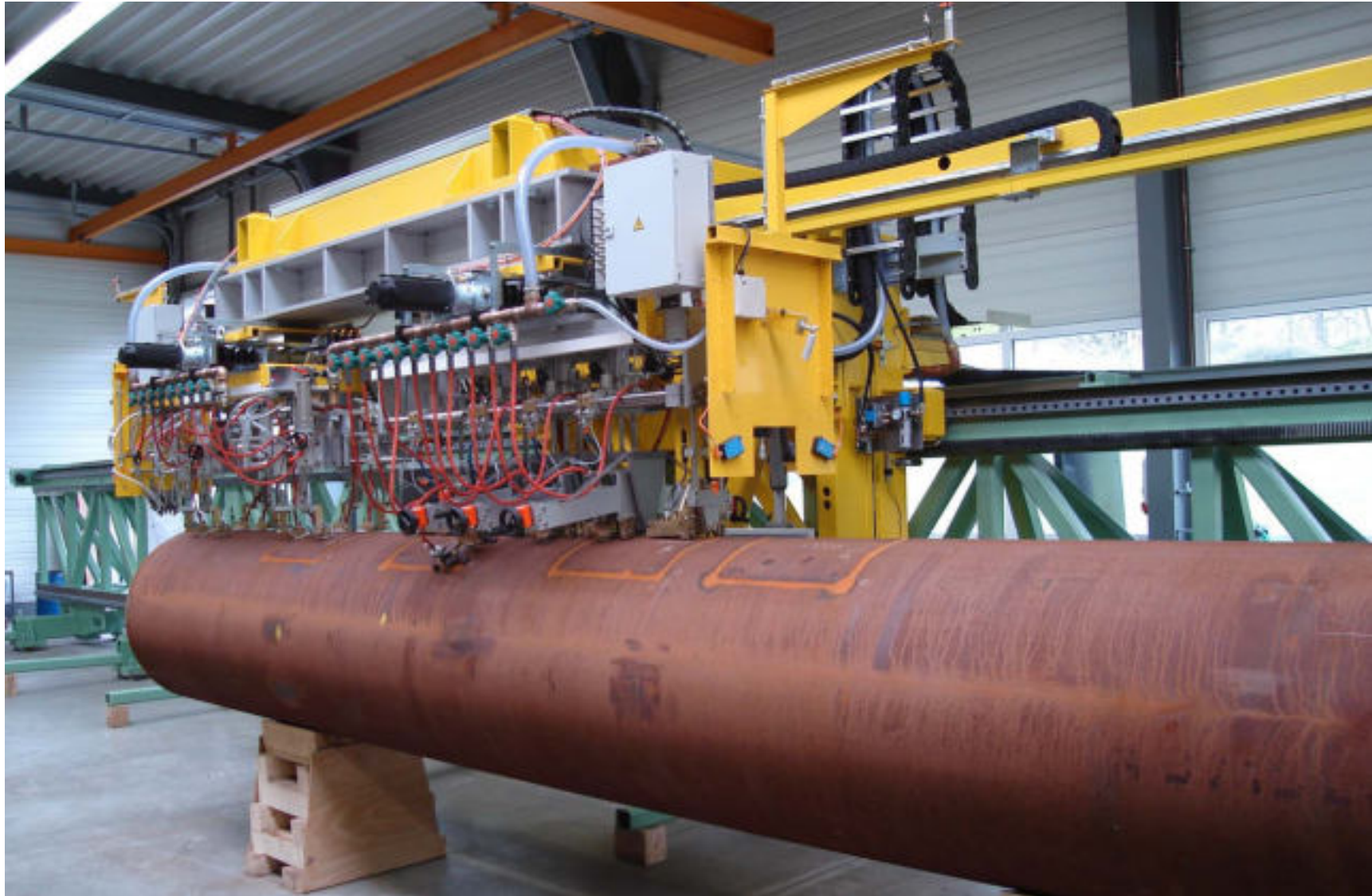
SNUL Prüfportal vor Expander Testing Portal before Expansion
