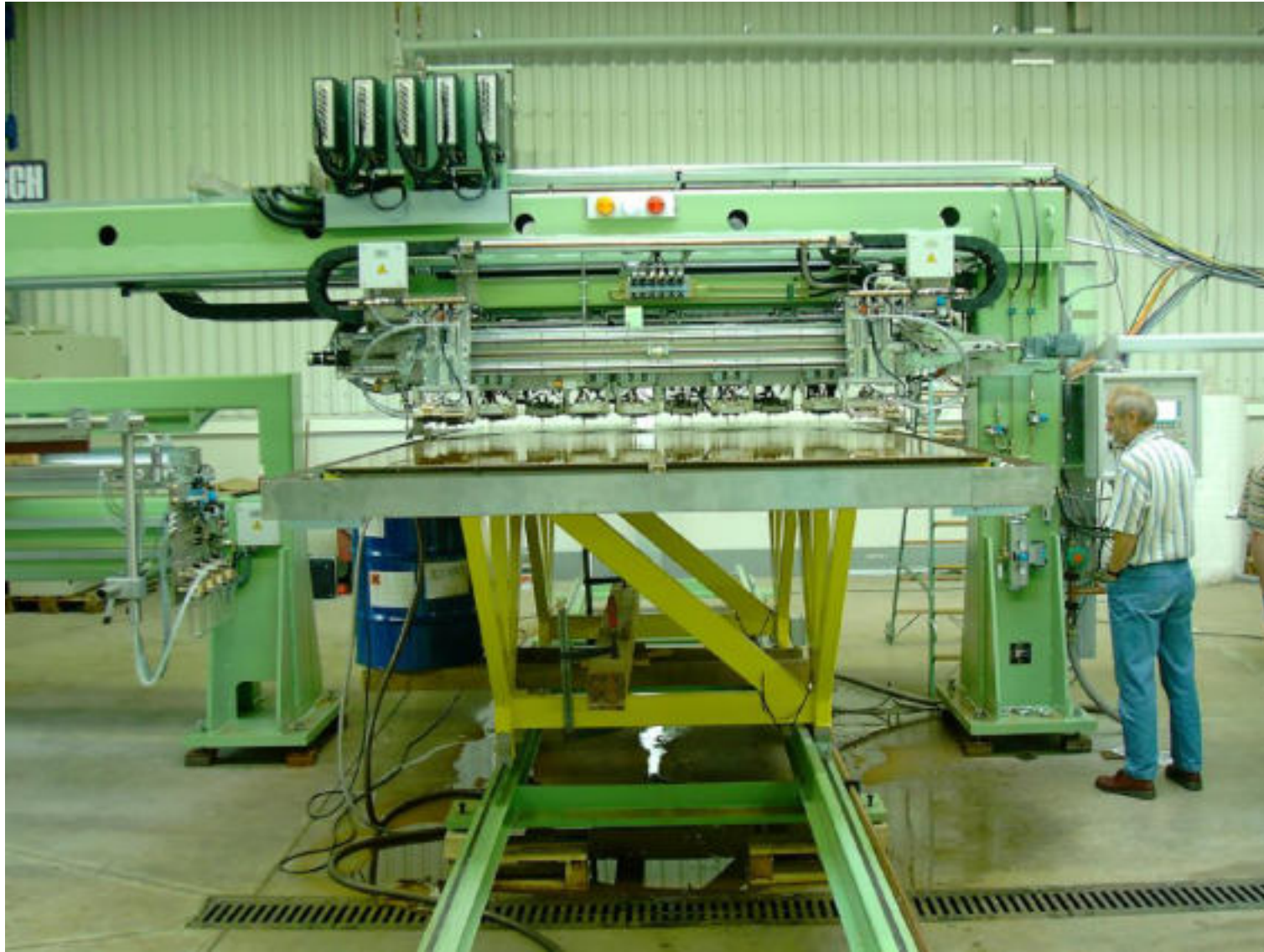
BAPS-Echograph1155 (37 probes) @ Baosteel China 2005
