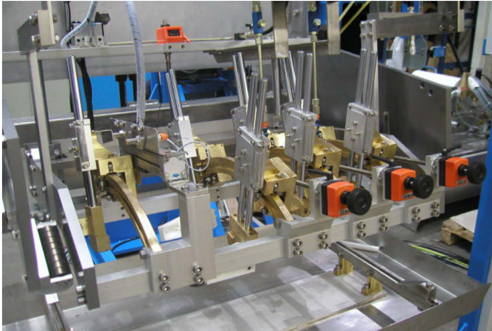
SNHF-Echograph1030-4L2DP1OSC (7 probes) @ SAFA Iran 2004
