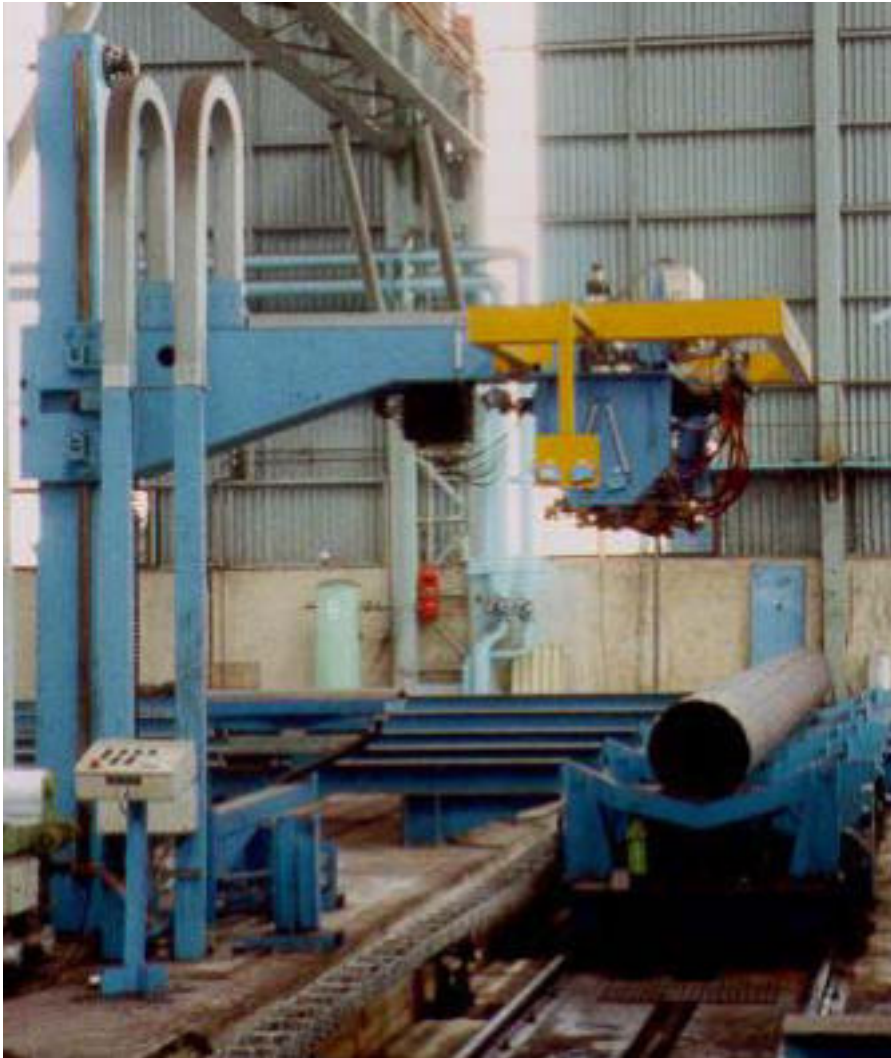
SNUL-Echograph: UP-Längsnaht LSAW-Pipe Testing
