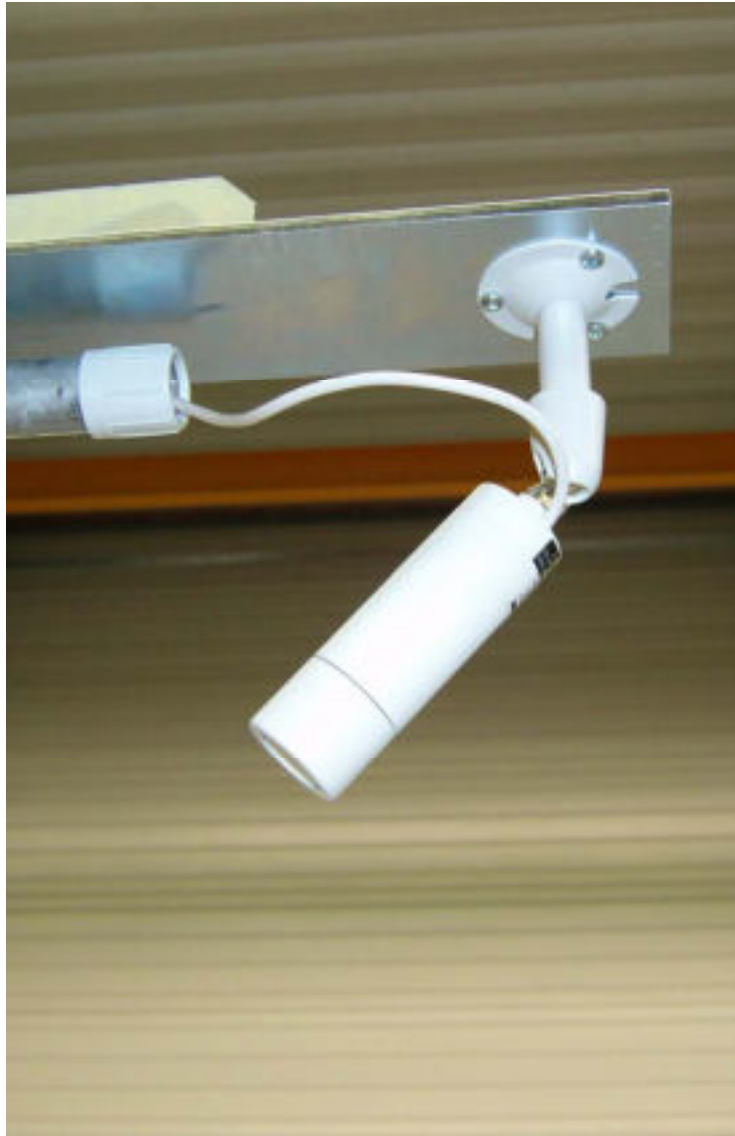
SNUL: Kamera & Monitor (Nahtfolger) Camera & Screen (Seam Tracking)
