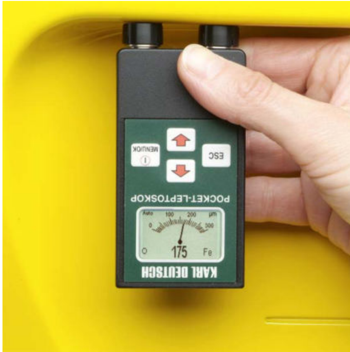
Pocket-Leptoskop: „Quasi-Analogue“ Measurement Display
