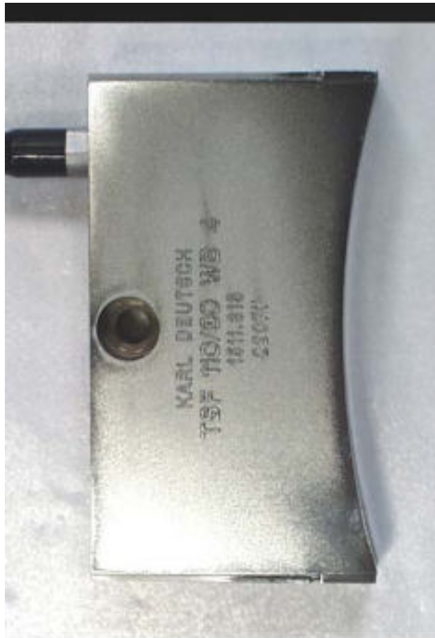
TSF 110/30 WB 4 ( f = 4 MHz, Line focus = 110 mm)
