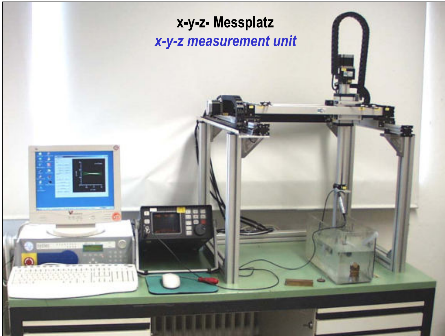
Schallfeld-Messung im Tauchtank Immersion Tank for Sound Field Measurement
