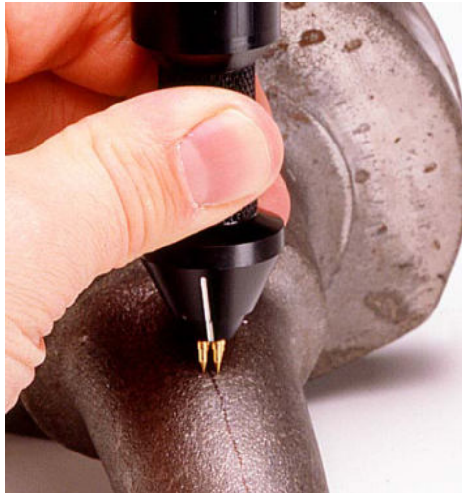
RMG Risstiefen-Messung RMG Crack Depth Measurement
