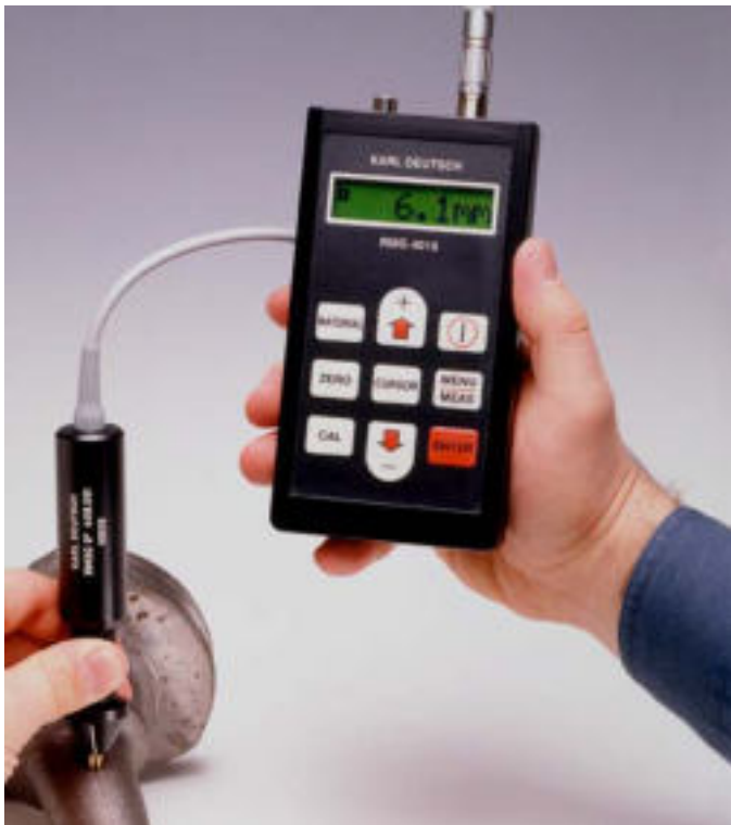
RMG Risstiefen-Messung RMG Crack Depth Measurement
