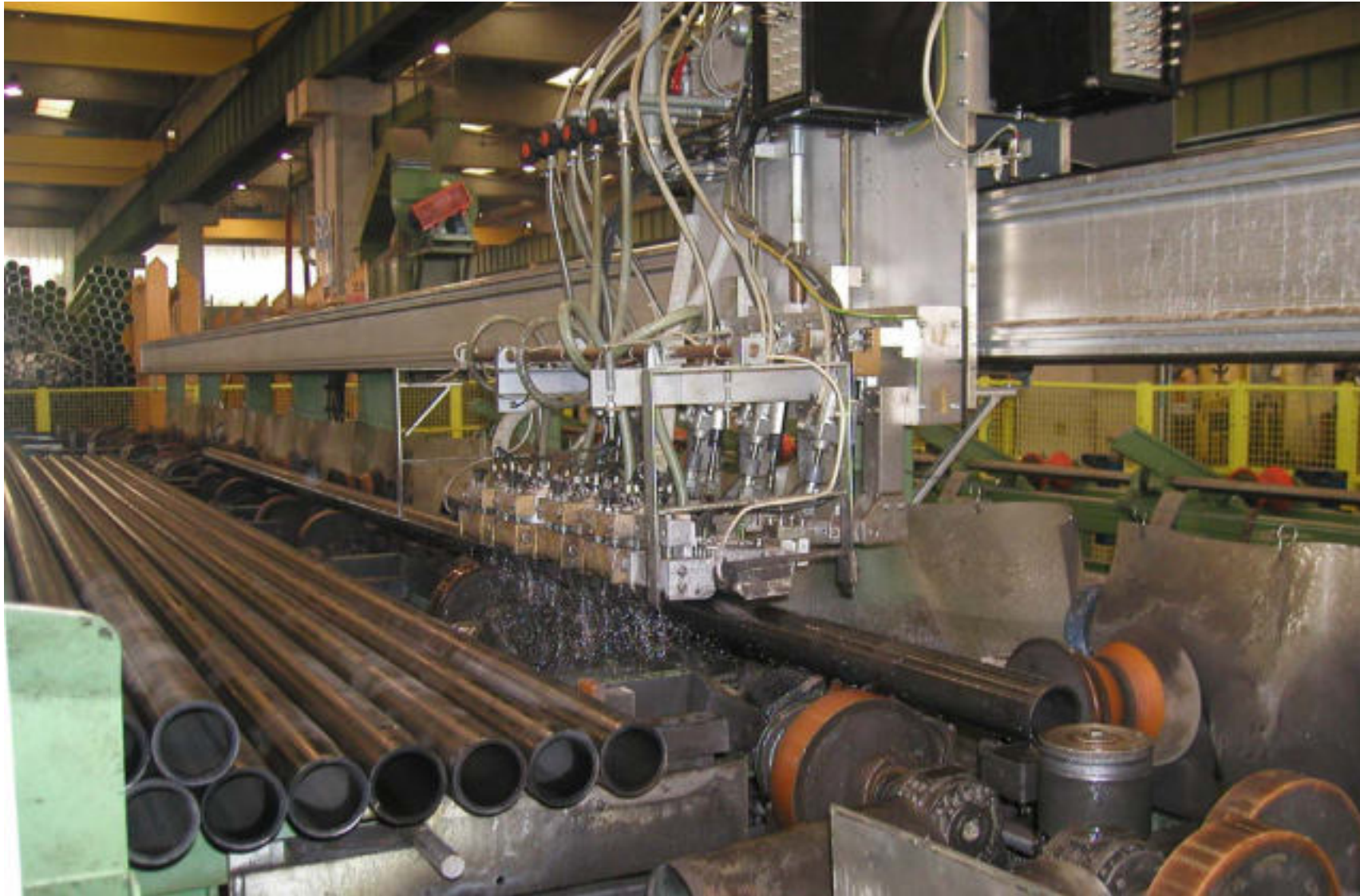
RPT.R-Echograph: Nahtlose Rohre Seamless Tube Testing
