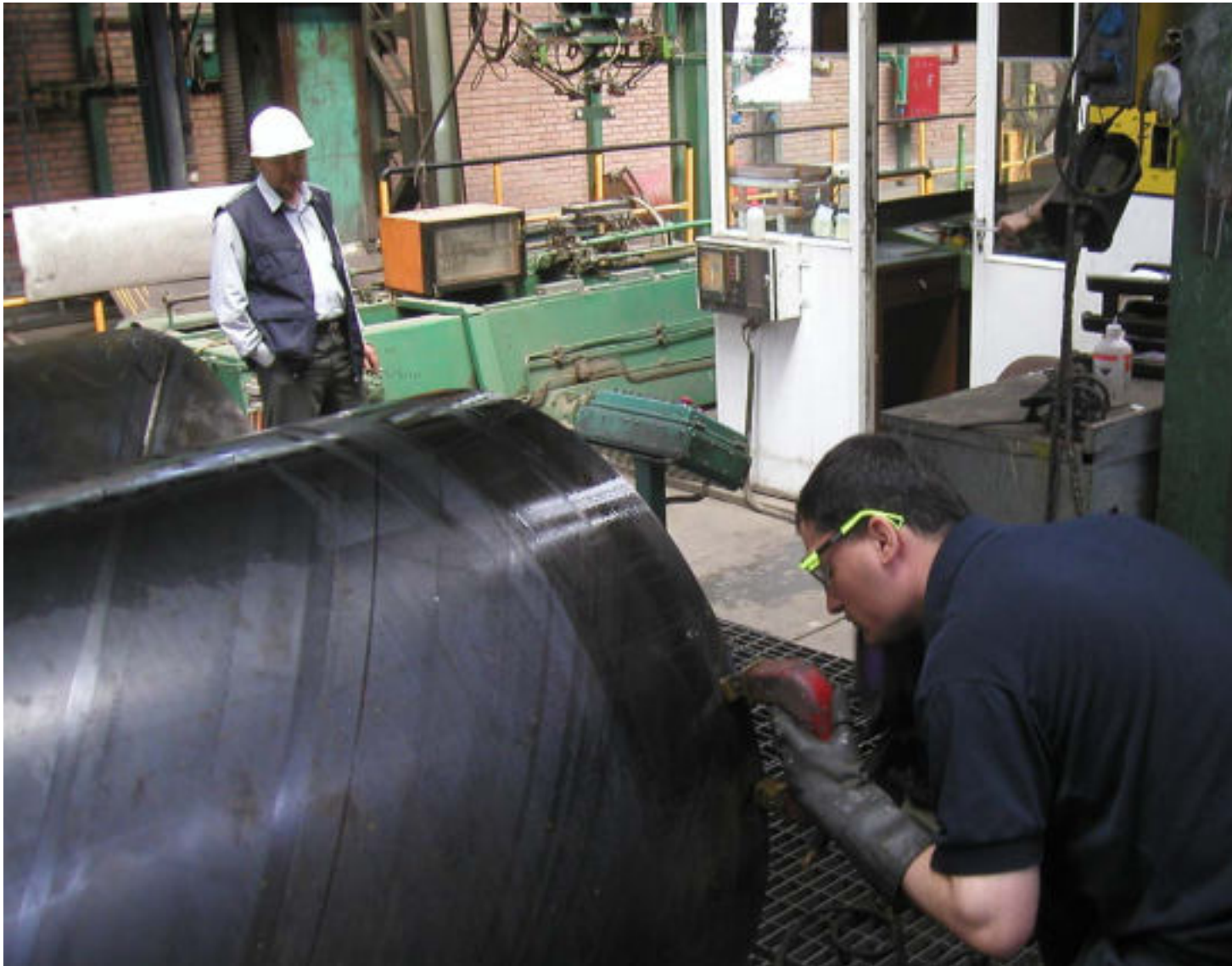
MP-Rohrenden-Prüfung Pipe End Testing (Magnetic Particles)
