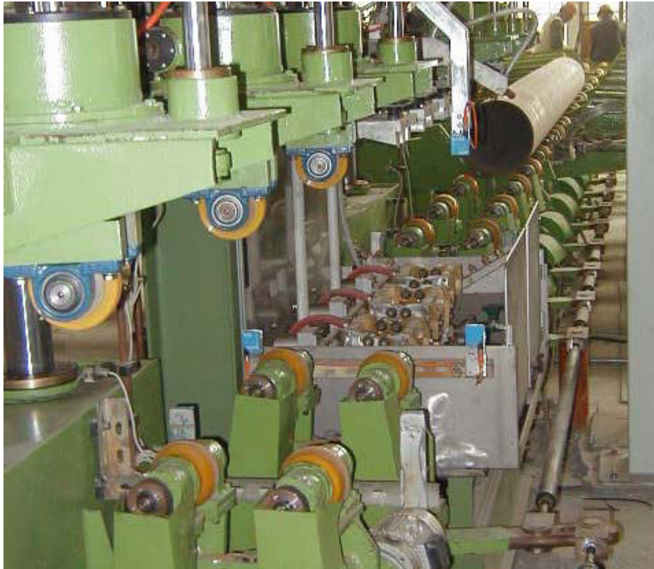
RPS.R-Echograph: Spiral-Rollgang Spiral Pipe Conveyor
