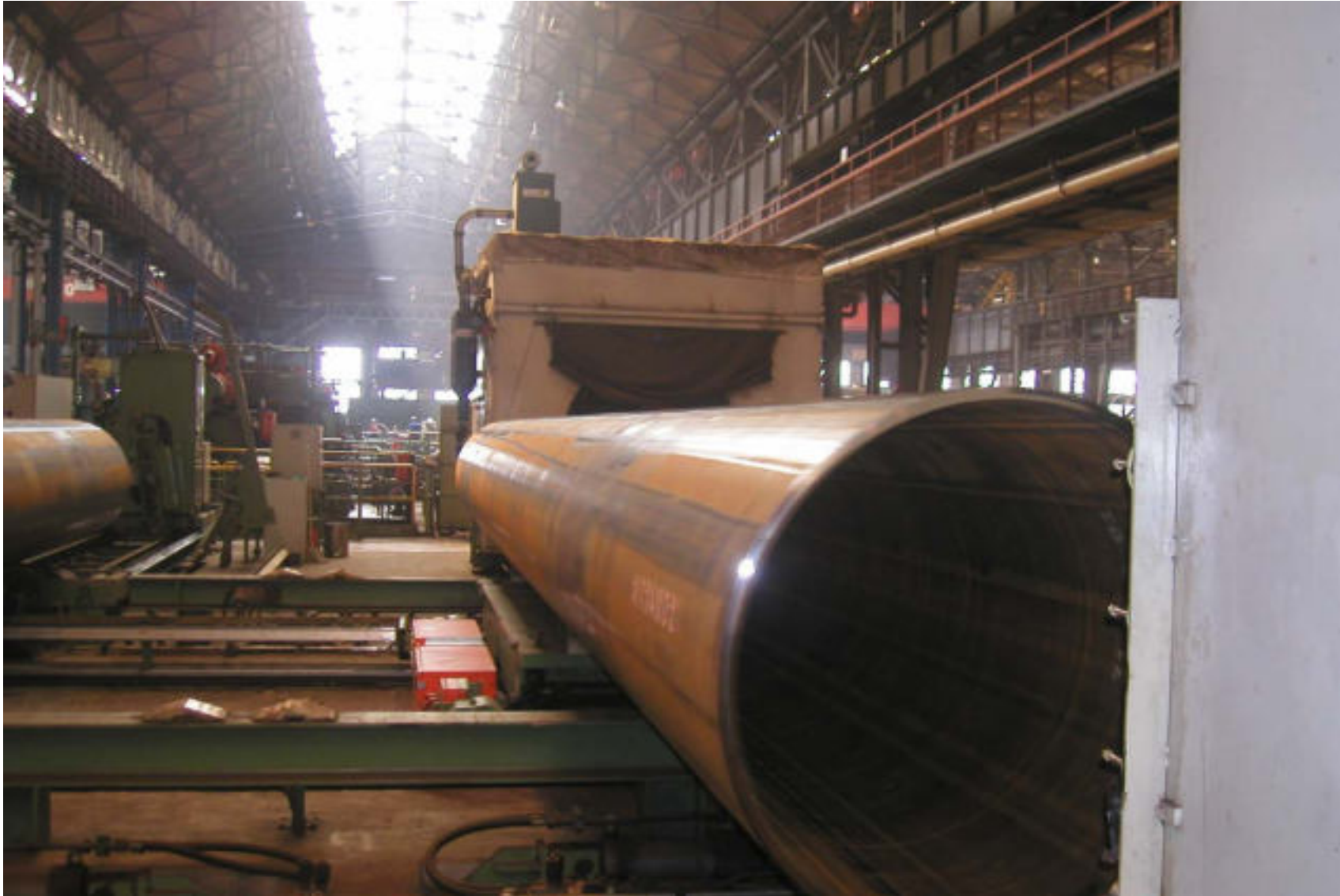
Rohrenden-Prüfung LSAW-Pipe End (@ Europipe)
