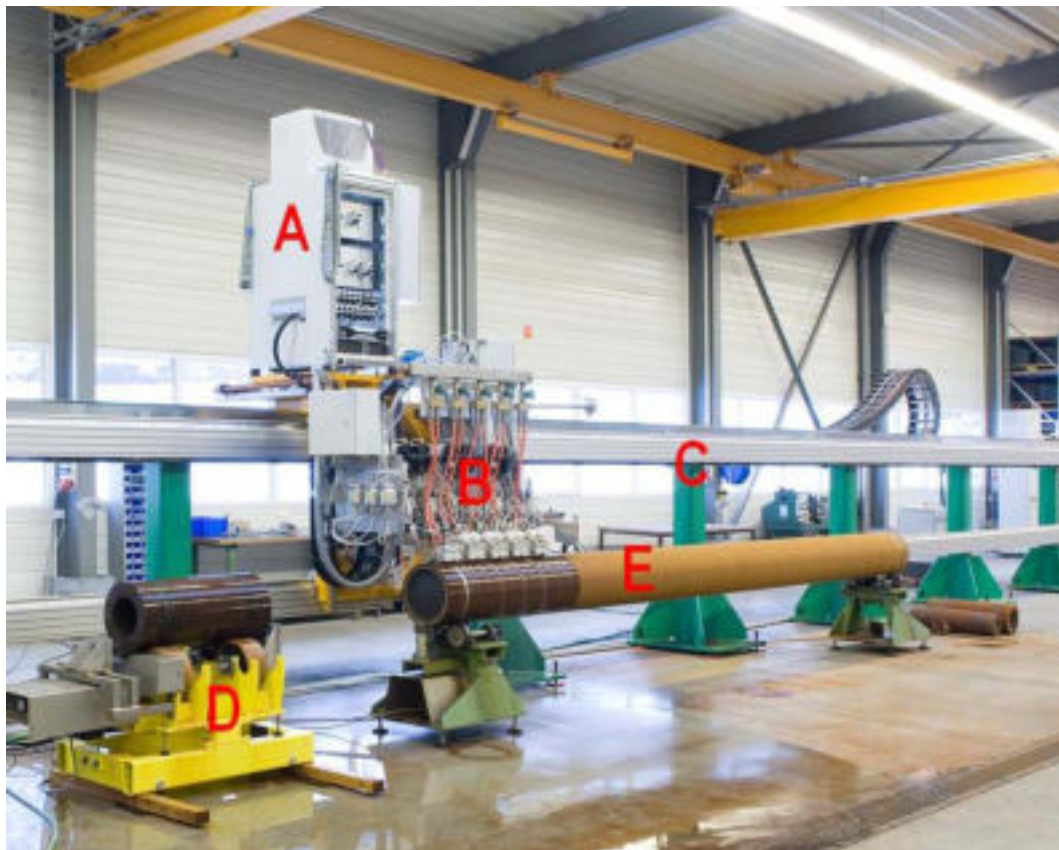
Figure Testing Mechanics. View of the testing machine in the systems workshop before shipment. A = testing electronics, B = probe holders, C = testing portal, D = calibration station, and E = production tube.
