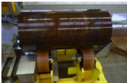
Figure Test Tube. (Provisional) calibration station with rotating device and calibration tube (406mm x 28mm).
