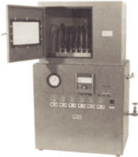
Coolant-circulating pressure system for testing automobile coolant hose using ethylene glycol solution at 270°F.
