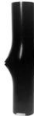
Polyethylene pipe sample after long-term hydrostatic testing, with localized ballooning and rupture
