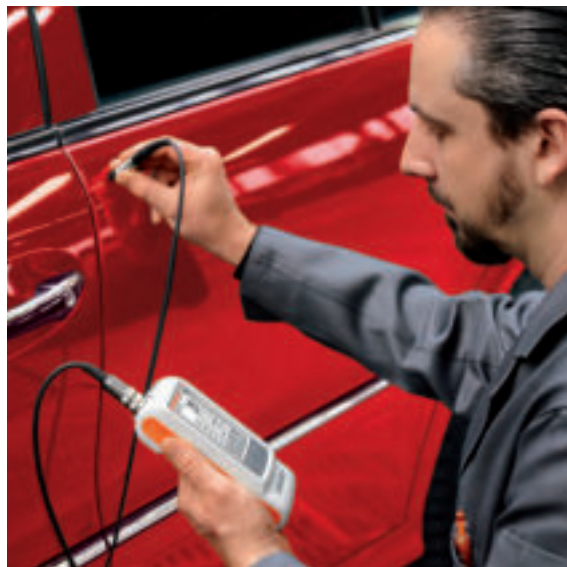
Measurement of auto body paint thickness using the Dual probe FD10
