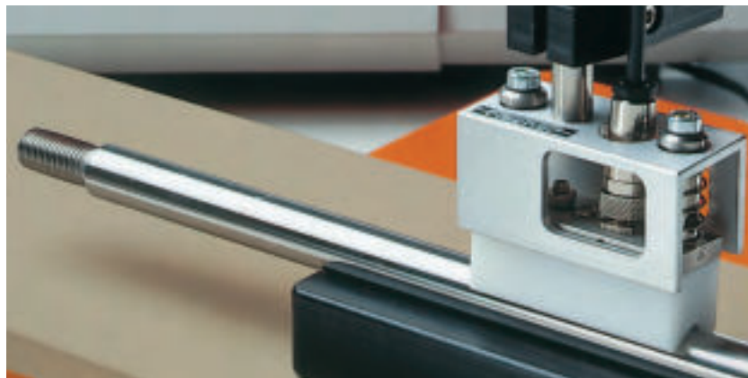
Automated measurement of the chrome coating on piston rods with the probe V2FGA06H
