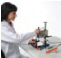
Measurements of anodized coatings on sleeves using the curvature-compensating probe FTD3.3, mounted into the support stand V12 BASE
