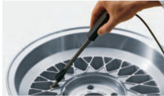
Measurement of the lacquer thickness on an aluminum rim wheel with the probe FAW3.3, mounted in the guiding device
