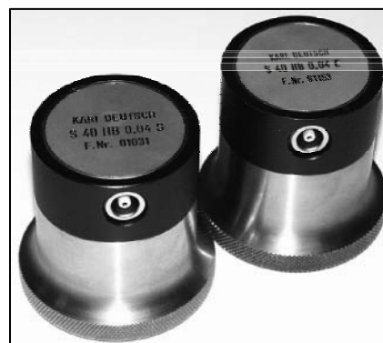
Pair of transmission mode contact probes S 40 HB 0,04
