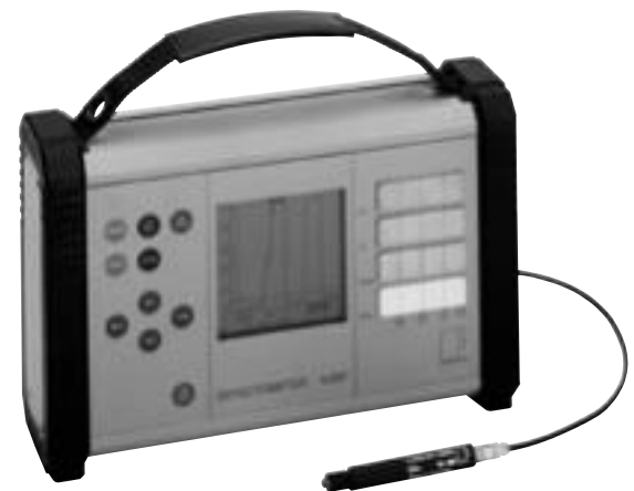
DEFECTOMETER 2.837 with probe
