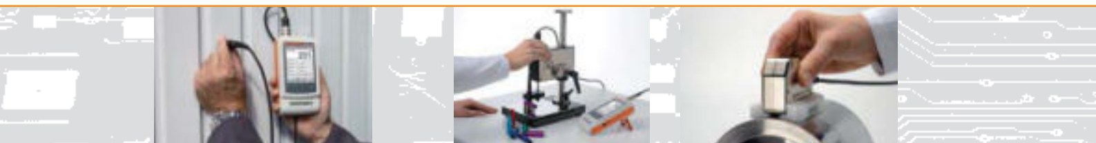
Measuring paint coating on steel
