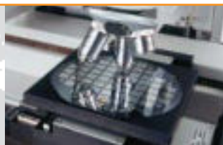
Wafer: Hardness determination on the gold coating
