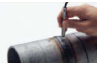
FERITSCOPE® FMP30: Ferrite content measurement on weld seams
