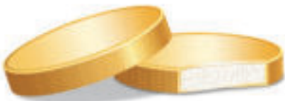
Schematic drawing of counterfeit coins with embedded powder of a tungsten-based foreign alloy and gold coating
