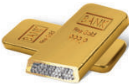
Schematic diagram of a counterfeit gold bar with embedded tungsten rods and gold cover
