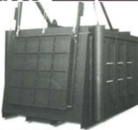
Front-loading box furnace, 2200°F (1204°C), for batch heat treating
