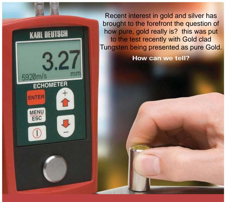
Tungsten or any Foreign Material insertion in gold bar & ingot can easily be uncovered by the use of the **Echometer** by Karl Deutsch of Germany. For Gold all foreign products have a different Velocity to Gold, taking this into consideration a quick and non-destructive thickness test of your Gold with the Echometer will show any irregular thickness reading straight away, with no impact on the sample.
