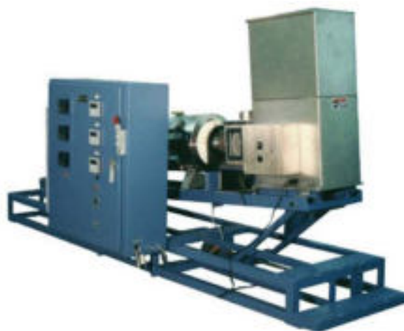
High-Temperature Rotary Calciner: Complete system including three-zone furnace, support frame with mechanical pitch adjustment, stainless steel hopper with vibratory feeder, rotary tube with agitator and speed control, and integrated control system for all components.
