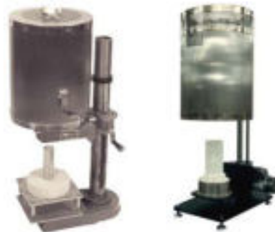
Specimen Loading Systems: Shown is a manual rack-and-pinion system (left) for raising and lowering a furnace onto a specimen and a motorized lift (right) for loading and unloading of specimens into a furnace.
