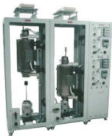
Dual-Station Computer-Controlled Carbon Reactivity Test System: Including split tube furnaces, reactor vessels, pneumatic lift system for specimen loading, and integrated temperature and gas flow control systems.
