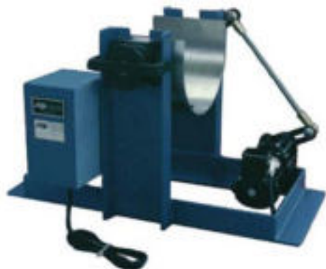
Tube Furnace Rocking Mechanism: Designed to continuously agitate material inside of a furnace tube through an arc of 22.5° at a rate of up to 15 cycles per minute.
