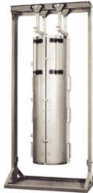
Vertical Support Stand with Rails: The sliding rail system on this structural support frame allowed each furnace half to move out of the way for unrestricted access to a vessel hanging inside the furnace.
