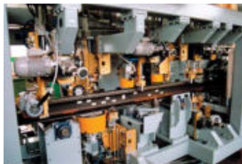
Eddy-current system for testing rails for surface flaws with rotating disks CIRCOSCAN® and shape-adapted segment coils
