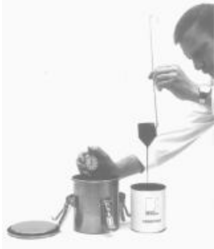
Fig 7 Flow cup in accordance with DIN 53211 for checking the color viscosity
