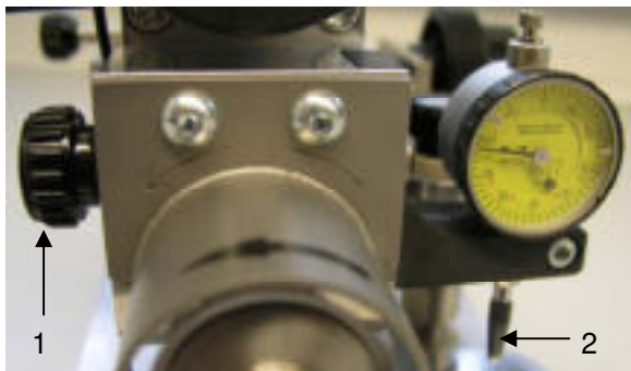
Fig 11 Level adjustment of dial gauge
