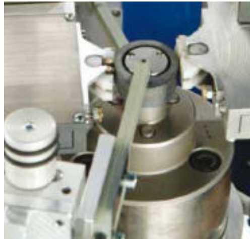
▲ Crack detection on individual cams with two testing probes on the contact surface and one testing probe on each face side.
