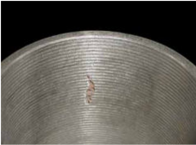
▲ Example of a surface defect located during automatic testing.
