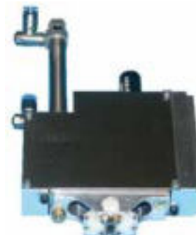
▲ MECA-PROBE for testing of excentric parts like individual cams or camshafts with a flat or abrupt contour.
