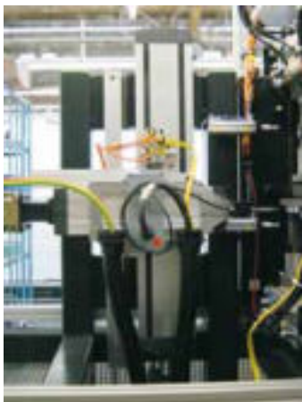
Detailed view: Numerically controlled traversing unit with eddy current probe. ▲
