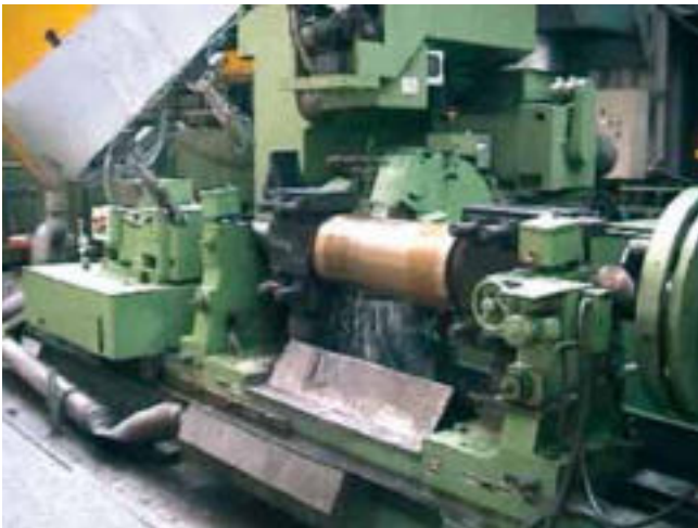
▲ Roll grinding machine within roll-shop with integrated eddy current testing.
