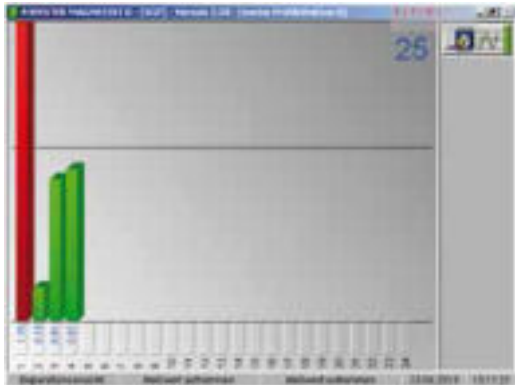
▲ At multi-frequency testing the results of up to a maximum of 24 single frequencies with the corresponding separation indices are shown in an overview.
