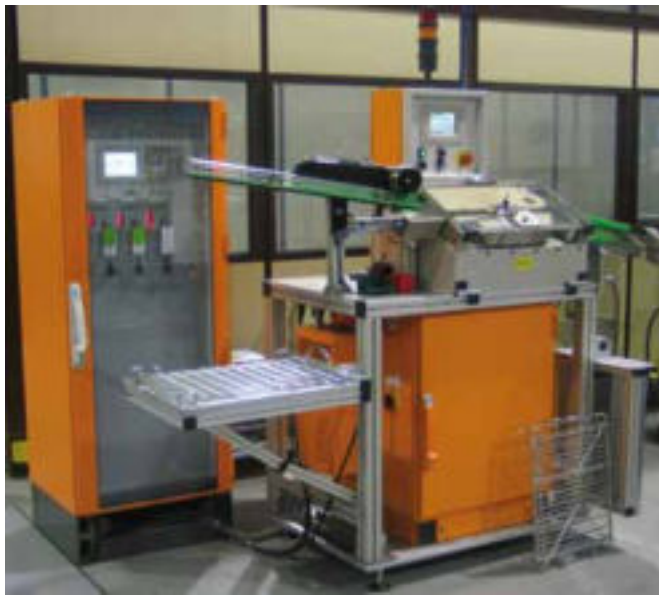
▲ Fully automated three-channel crack test system (Roto-Scan) with manual loading of the test piece buffer or line integration.
