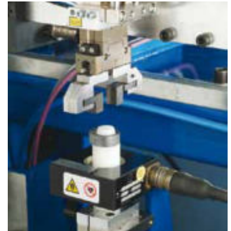
▲ Microstructure testing is additionally carried out on a separate station with an encircling MAGNATEST testing coil.
