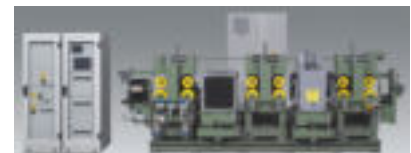
Fu Shun, China: Test Section for bars with CIRCOGRAPH Ro 130 + DEFECTOMAT channel M 140 + EMAG F
