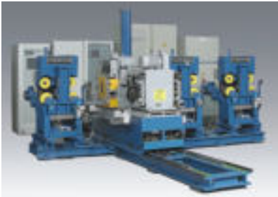
Stahlwerk Südwestfalen, Germany: Test Section for bars with CIRCOGRAPH Ro 130 + MAGNATEST DHZP + space for US
