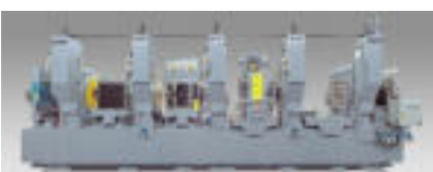
voestalpine Tubulars, Austria: Test Section for tubes with DEFECTOMAT M 170 + TRANSOMAT TR 180 + ROTOMAT Ro 180 + laser diameter measurement + EMAG F + space for US by General Electric
