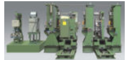
Hengyang, China: Test Section for tubes with ROTOMAT Ro 440 + TRANSOMAT TR 440 + special EMAG
