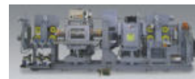
Gerdau, Brazil: Test Section for bars with US by Nutronic + CIRCOFLUX Ro 100 + MAGNATEST DHZP + laser diameter measurement
