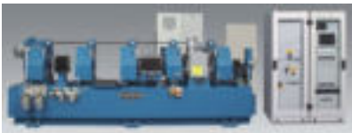
Stahlwerk Judenburg, Austria: Test Section for bars with MAGNATEST DHZP + CIRCOGRAPH Ro 65 + DEFECTOMAT channel M 90 + space for US + EMAG F
