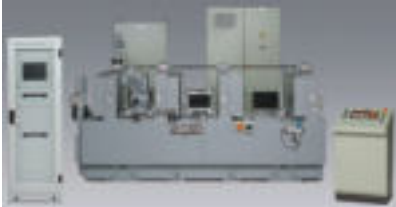
Saarblankstahl, Germany: Test Section for bars with CIRCOGRAPH Ro 35 L + DEFECTOMAT channel M 40 + EMAG M
