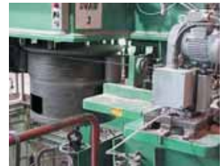
▲ Testing steel wires directly in the bull-block machine with CIRCROGRAPH rotating head.
