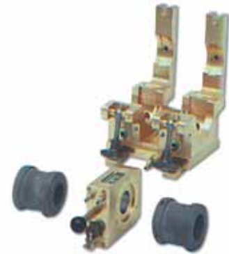
The T 60 sensor system has a modular design. Special-purpose guide elements steady the wire and ensure that it is guided as centrally as possible. Water-cooled coils and guides are available from 5 to 65 mm.
