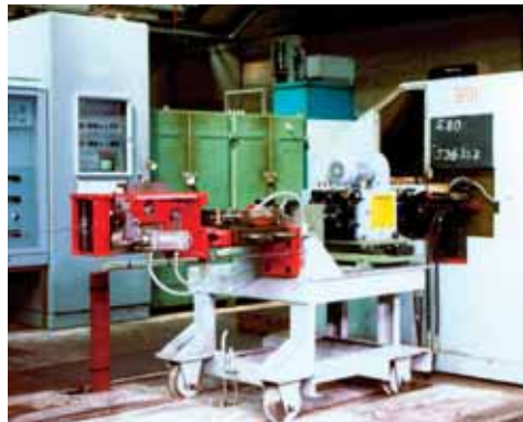
▲ CIRCGRAPH tests prior to the bolt or screw press. Finished parts made of flawed wire sections are segregated off downstream of the press.
