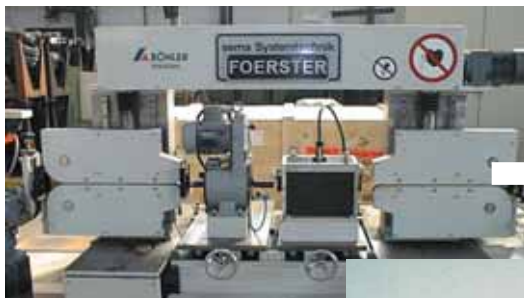
▲ A compact testing section with belt guidance allows testing of polished stainless steel bars in the dimension range 2 – 20 mm with high flaw sensitivity even at a speed of 2 m/s.
