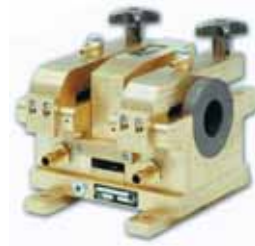
The T 60 sensor system has a modular design. Special-purpose guide elements steady the wire and ensure that it is guided as centrally as possible. Water-cooled coils and guides are available from 5 to 65 mm.
