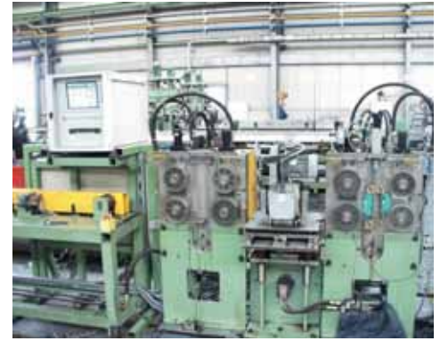
▲ Test of steel wire by Ro 35 L integrated in a cut-to-length-line.
