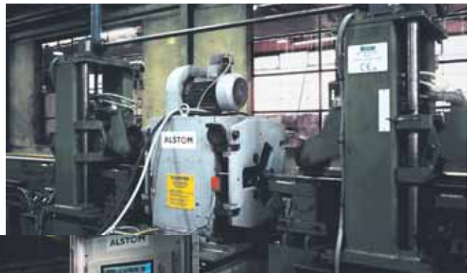
▲ The low-vibration and precise material guidance ensures reliable and reproducible results when testing bright steel in bar form with CIRCGRAPH DS + Ro 65.
