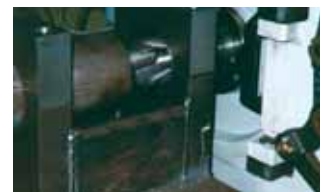
▲ The special-purpose, funnel-shaped guide system of the Ro 65 facilitates exit and entry of the leading edge of the wire and trailing edge of the wire, in particular in the case of large dimensions.
