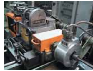
▲ Test of steel wire by Ro 14 and M 22 in recently installed Schumag drawing machine 0B.
