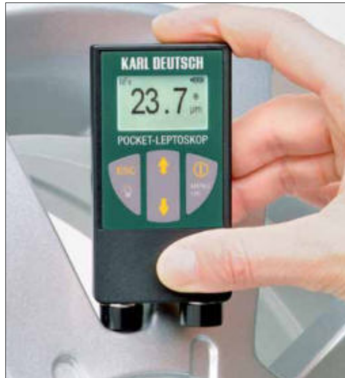
Compact gauge with integrated sensor (Pocket-LEPTOSKOP® 2026)
