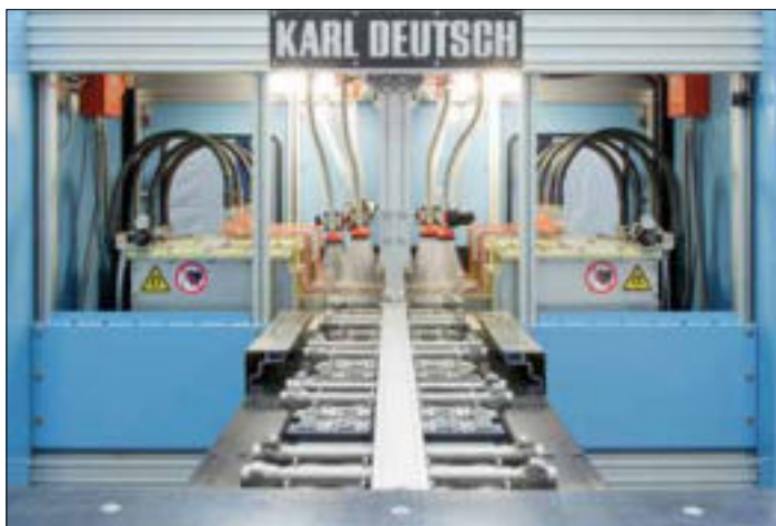
DEUTROMAT with chain conveyor, 8 components per cycle
