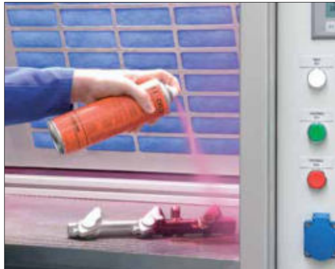
Testing of a forged component with red penetrant
