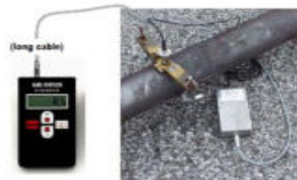
Fig. 2: Measuring location on pipe with permanently installed wall thickness probe (middle), on-site wall thickness electronics (right bottom) and remote ECHOMETER unit as host station and/or data output (left). The cable length can range from 100 m (RS 232 serial interface) up to 1200 m (RS 485 serial interface).
