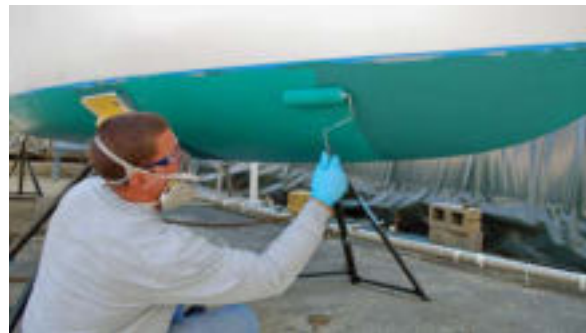
Fig. 2: Applying a new coating requires consistent thickness readings.
