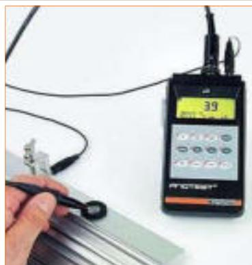
FISCHER ANOTEST® YMP 30-S tests the sealing quality of anodic coatings on aluminum, which is an important factor for weather resistance. It measures the admittance Y of the anodic oxide film in accordance to DIN EN 12 373-5 and ASTM B 457-67.
