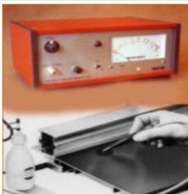
FISCHER Anotest. Measures the sealing quality of Anodic coatings. Still in use by customers and still repaired and calibrated by KK&S Instruments.
