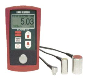
The new generation of the ECHOMETER series can now measure wall thickness and sound velocities in one instrument and therefore offers many advantages for the operator. This innovative dual-use Echometer has been re-designed by Karl Deutsch the well-known supplier of testing instruments and testing systems in Germany.
