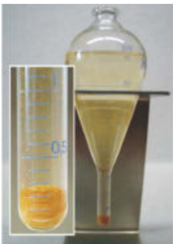
Fig. 4: Measurement of magnetic particle concentration according to AMS 3044 / ASTM D 56
