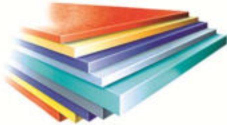
Figure 1: Layered coating structure of coated steel sheets used for the manufacture of roofing: steel base material (green), zinc coating (light blue), protective layer (dark blue) and 2 layers of Paint (yellow, red).
