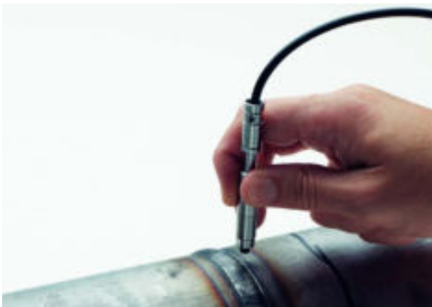
Fig.1: Measuring the ferrite content of a weld seam with FERITSCOPE® Helmut Fischer FMP30 and the probe FGAB1.3-Fe
