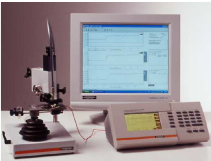
Figure 2: With the measurement system COULOSCOPE ® CMS STEP the potential development during the detachment of a layer can be depicted and analyzed.
