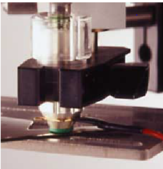
Figure 3: Deplating cell with new, conically formed reference electrode.
