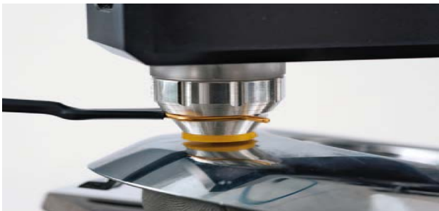
STEP Test measuring cell placed on a specimen
